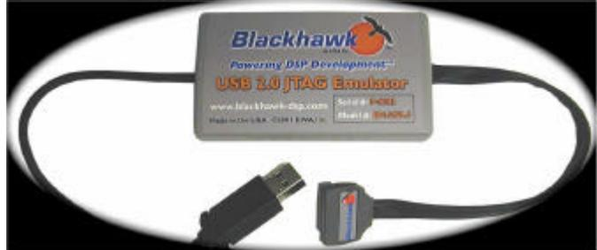
The Blackhawk™ USB 2.0 JTAG Emulator is the interface between a graphical user interface (GUI) debugger running on a laptop or PC and the target DSP. The JTAG, scan path - based emulation (IEEE 1149.1) provides developers with non-intrusive target architecture. The target hardware requires only a 14-pin header connected to the scan path pins of the DSP chip.
